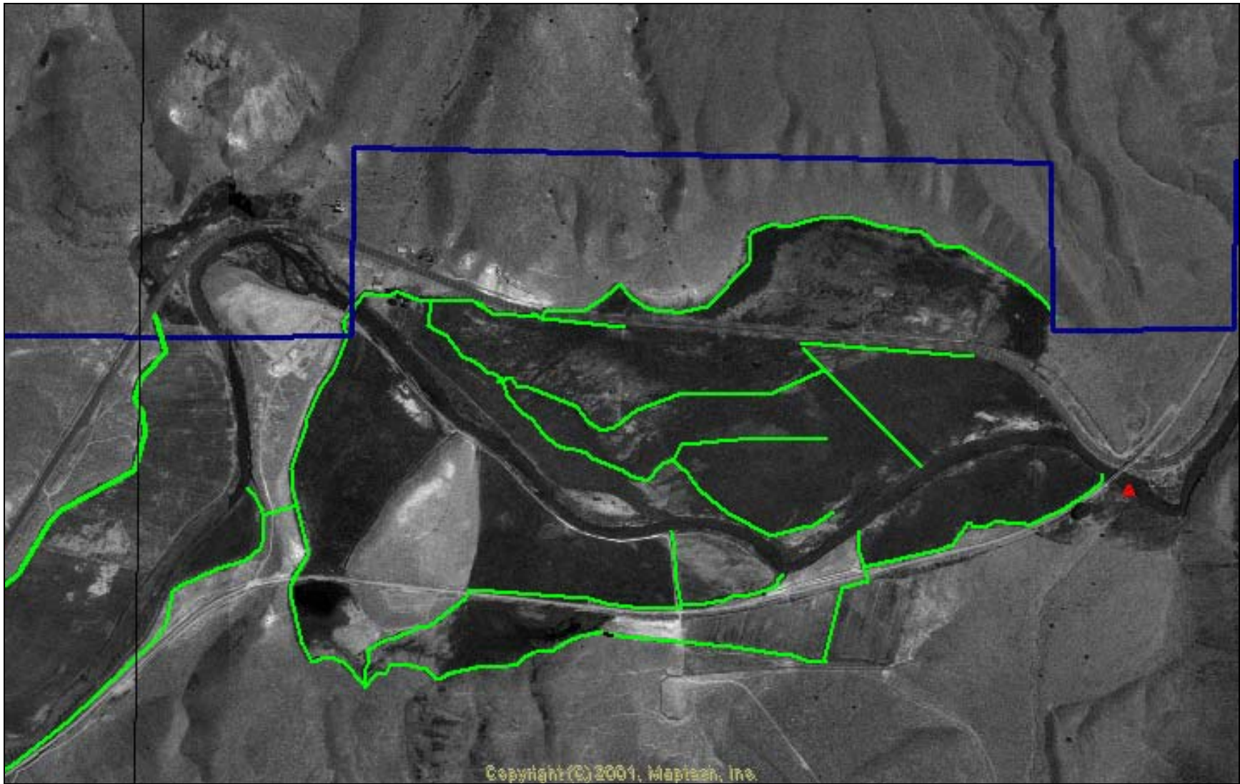
Figure 25. Irrigation canals and ditches (green lines) on middle section of Malheur River/Black Canyon Unit.
